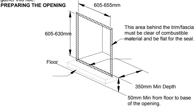
The front face and the base of the fire opening must be flat to ensure that a good seal is formed between the rear and base of the appliance and the chimney to avoid any reduction of natural draught.
